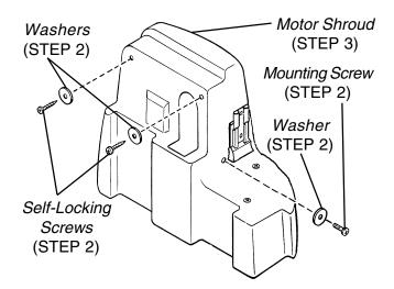
FIGURE 3 - REMOVING THE MOTOR SHROUD
